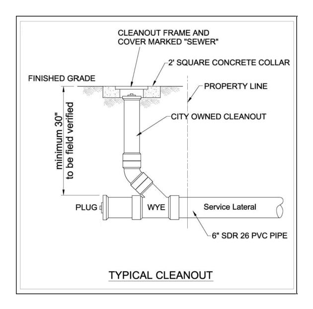
The City requires that the Sewer Laterals be constructed in accordance with AirVac recommendations. Pressure rated pipe (Schedule 40/SCH80 or SDR 21/SDR26 PVC) is required for the Laterals because from time to time, your Lateral may be exposed to conditions which could cause non-pressure rated pipe to collapse.
