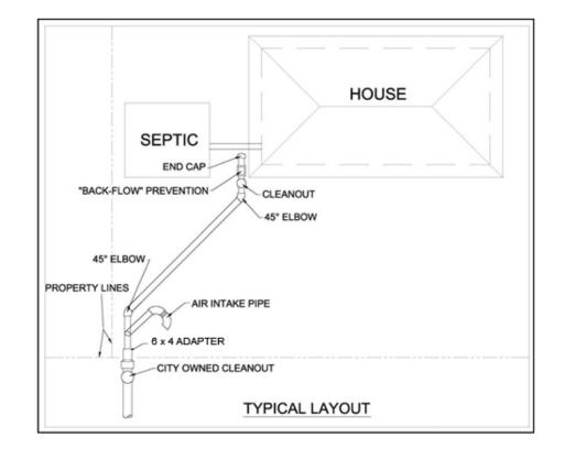
The following drawing shows a typical layout and trench detail.
